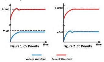
As shown in figure one, when the DUT requires reducing voltage overshoot during test, such as supplying power to a low-voltage processor or FPGA core, voltage priority mode should be selected to obtain fast and smooth rise voltage.
