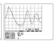
Total Area Comparison By calculating the area between DUT and golden sample, and compare the difference. Judge the energy cost by analyze the wave.
