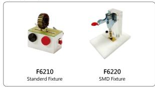
Standard fixture F6210 for measuring inductance, optional fixture F6220/ F6240 for measuring SMD inductance.
