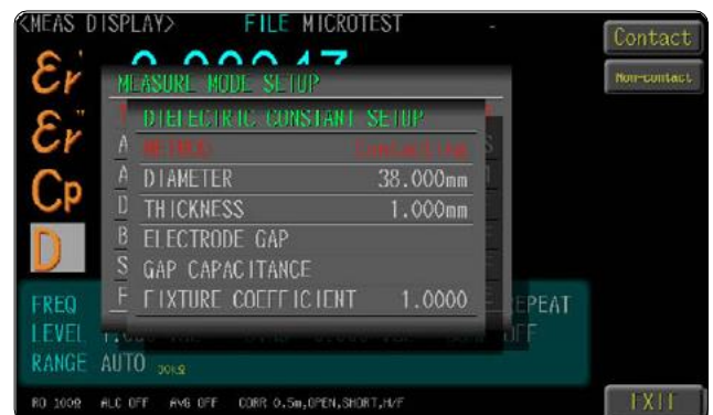
Dielectric Material Test Fixture (FX-000C7) Using the dielectric material test fixture for measuring PCB board or ceramic board. 6630 built-in formula to directly calculate the material dielectric value \epsilon_r' , \epsilon_r'' .
