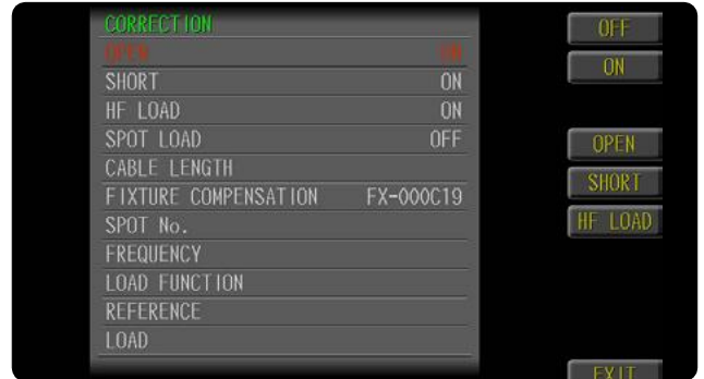
Correction Before measuring the DUT, you should select "Correction" button to do open, short, and HF Load or SPOT Load correction.
