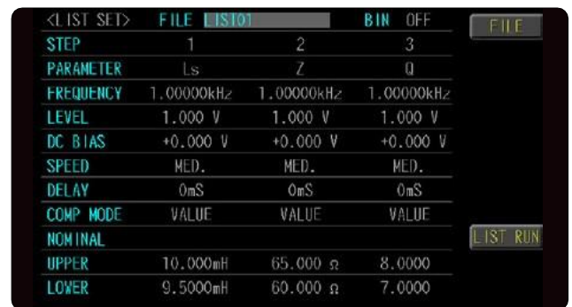
List Mode 50 groups of list mode setting (Each group contains up to 15 steps).
