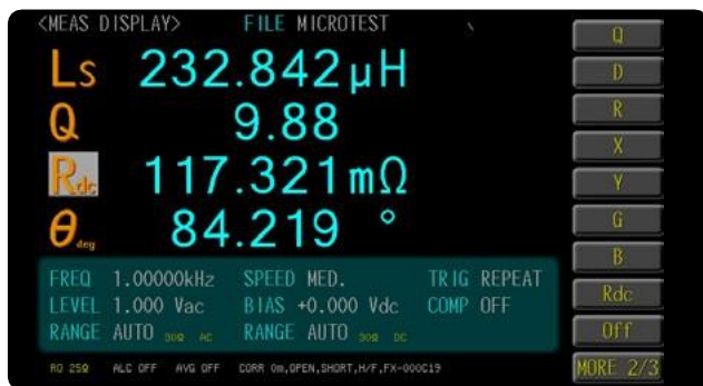
Measure Inductor (DCR) Inductor coil turns and winding materials will affect DCR value. The key parameters for inductor are Ls / Lp / Q / SRF / DCR.
